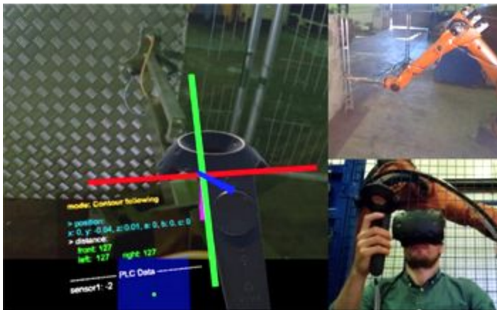
Operators view inside the VR, Immersive 3D view provides intuitive interface to control the robot.
